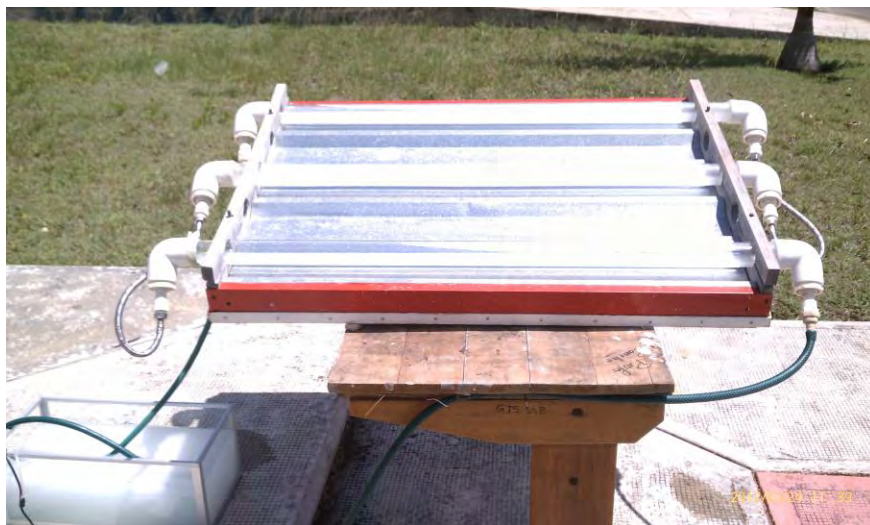
Figura 15. Reactor solar tubular.
